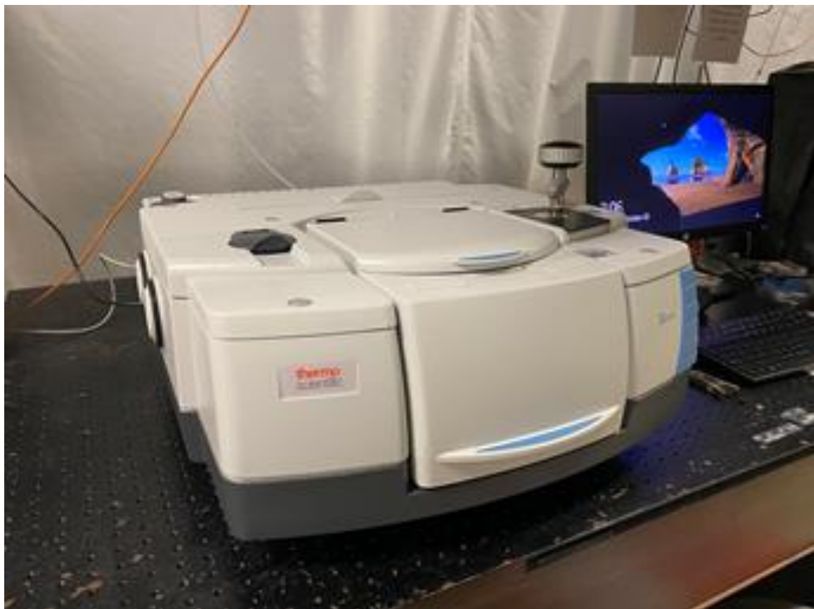
Obr. 3. Thermo Nicolet – príklad laboratórneho FTIR spektrometra (zdroj: https://mrl.illinois.edu/facilities/equipment/thermo-nicolet-nexus-is50-ftir )
